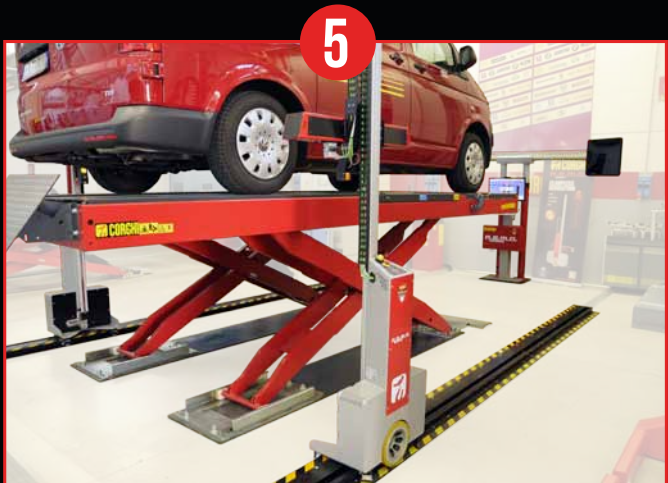
Possibility of reading even when the lift is raised
